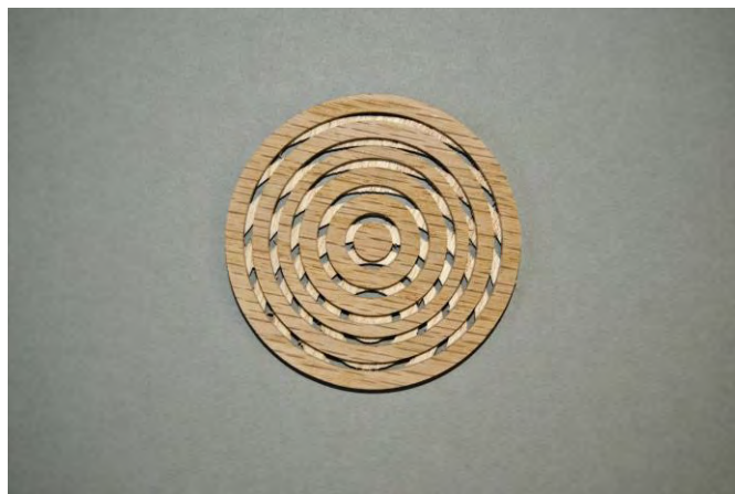
Figure 23 – The Resultant Lattice Pattern Insert (Pattern #7)
