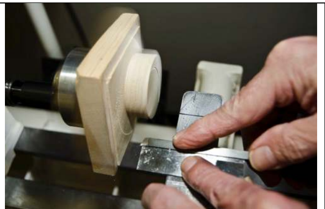
Figure 17 – Use the square as a guide for the skew to make a shallow cut, etching where the cut element is located on the pendant face
