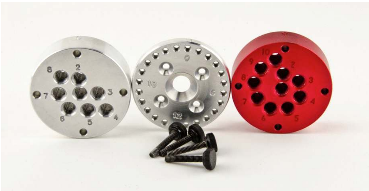
Figure 1 – The Richard Joyner Pendant Chucks – the original 8-Hole version on the left, the newer 10-Hole version on the right, with an index plate between them.
